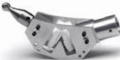
Ord.No. 1054 50° gearbox articulated joint / claw one side for tail boom
