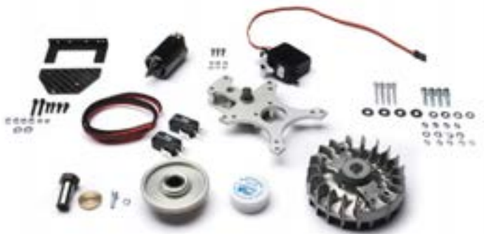
ORD.NO. 1023/5 on-board electric starter for G230/G240, 9.6 V, including: • starter motor with pinion gear Ord.No. 1023/9 • base plate and reduction gear stage incl. freewheel • modified fan • servo with switch adaptor to control the start-up • safety switch (must be used with the throttle servo to prevent starts above the low stick positio)
